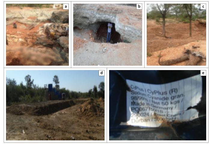
FIGURE 2: Artisanal mining at the Sutherland goldfield: (a) Fine gravel digging operations, (b) hazardous excavation at Louis Moore Mine, (c) the impact of excavations on trees around New Union Mine, (d) an abandoned cyanide heap leaching setup (e) and an empty container of the leaching chemical used.
